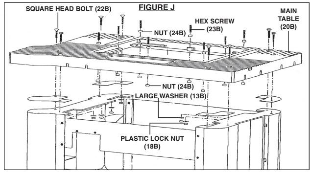
4. Screw a Nut (24B) downward on each of the *eight* Hex Screws (23B). Insert the Hex Screws downward through the *eight* mounting holes located on the Main Table (20B). Make sure the Nuts are <u>above</u> the mounting holes. Then, screw a Nut (24B) upward on each of the eight Hex Screws to secure the Hex Screws to the Main Table. **(See Figure J.)**
